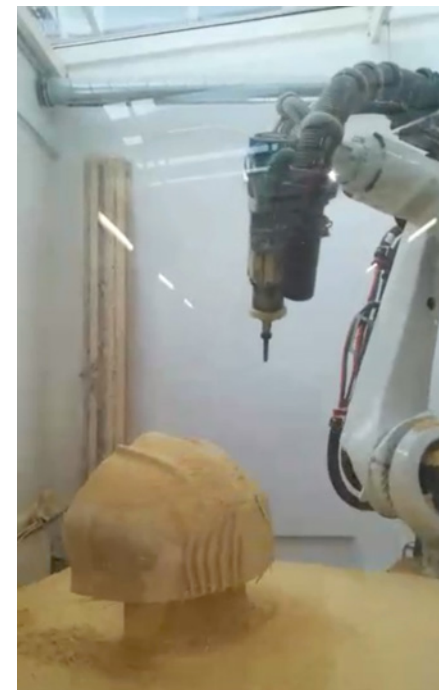
Figure X. Kuka robot and part of the Intelligent Guerrilla Beehive during fablab building in collaboration with the University of Applied Arts, Vienna.
